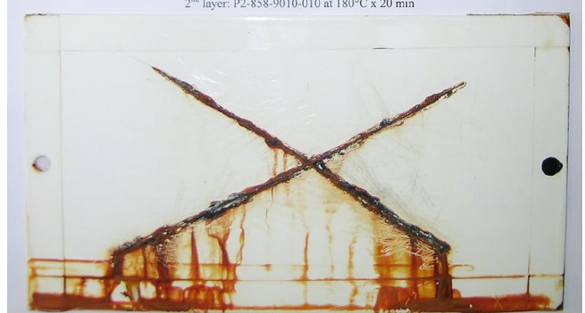
EY-658-7300-001 + P2-858-9010-010 on Zinc Phosphate Panel After 5.000 hours of Neutral Salt Spray (ISO 9227)
