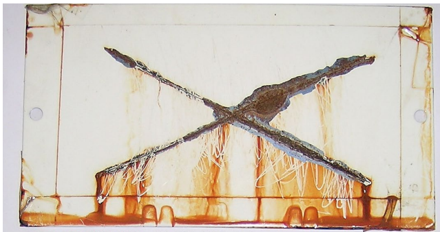
EZ-658-7300-010 + P2-858-9010-010 on Iron Phosphate Panel After 2.000 hours of Neutral Salt Spray (ISO 9227)
