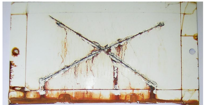
EZ-658-7300-010 + P2-858-9010-010 on Zinc Phosphate Panel After 5.000 hours of Neutral Salt Spray (ISO 9227)
