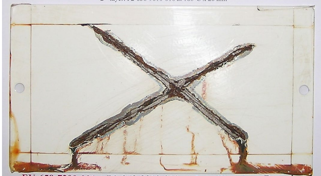
EY-658-7300-001 + P2-858-9010-010 on Iron Phosphate Panel After 2.000 hours of Neutral Salt Spray (ISO 9227)
